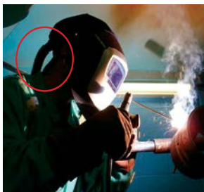
A respirator protects this welder.
