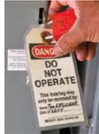
A machine being locked and tagged out
