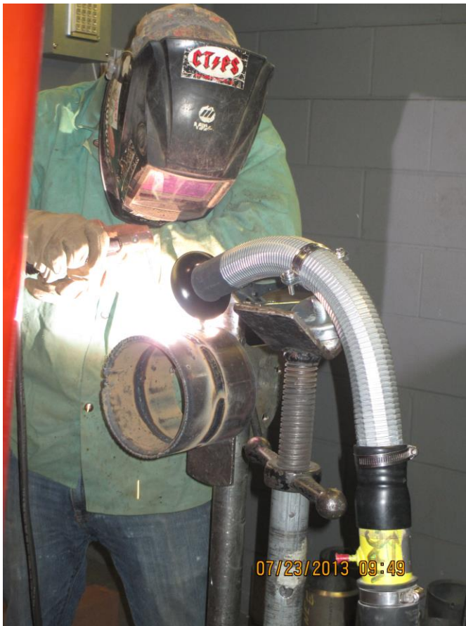
Figure 3: Welding carbon steel with LEV
